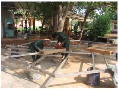
In the Metal Workshop the stain less steel support structure for the stage takes shape
