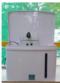
At Talam, CSR, we have developed an automatic hand sanitizer dispenser in-house at low cost, by modifying the standard water purifier box (the outer plastic body) to cut down costs.
