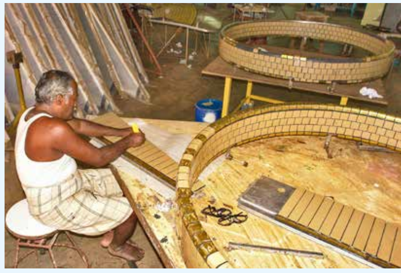
The creation of all the golden tiles for the discs and doorway shields was carried out in the Matrimandir workshops during the period from 1995 to 2007.
