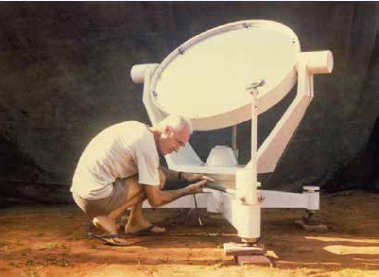
Piero Ciconesi, who guided every detail of the construction for the first 20 plus years, designed a heliostat to catch the sunray to be directed onto the globe in the Inner Chamber from the top of Matrimandir.
